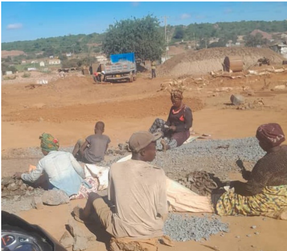
◀ Figure 3: Women engaged in manual crushing and sorting of rocks at Namba Tano site in Mwakitolyo (Photo by TAI, 2025).
